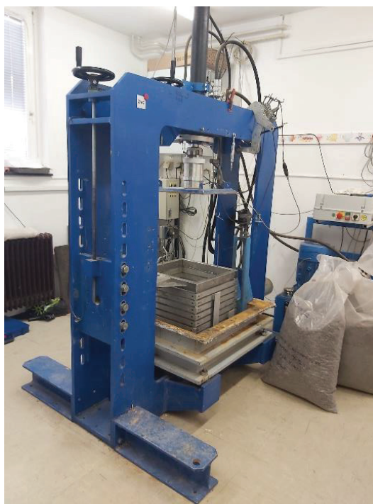
Fig. 4: Large-scale Triaxial Apparatus (ZAG Laboratory, Ljubljana, Slovenia)
