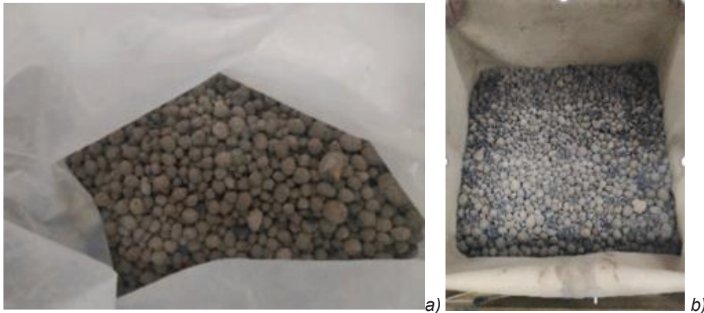
Fig. 5: Expanded clay aggregate material a) before installation, b) after testing, exposed to damage
