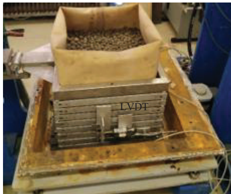
Fig. 6: LVDT sensors for strain measurements
