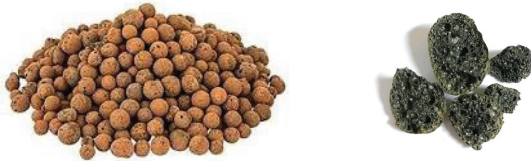
Fig. 2: a) Expanded clay aggregate; b) Interconnected different sizes of air-filled cavities
